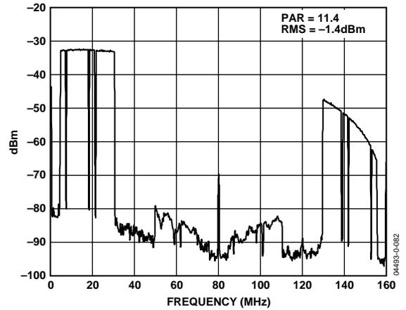
Figure 37. Wideband Spectral Plot of 111-Carrier OFDM Test Vector
