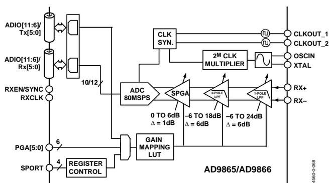
Figure 68. Functional Block Diagram of Rx Path
