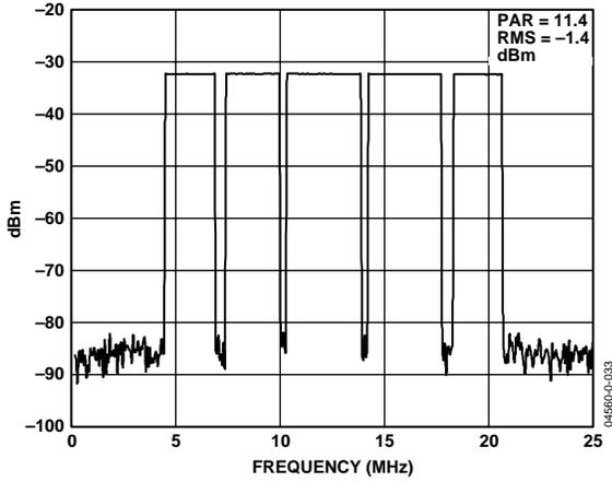
Figure 33. Spectral Plot of 84-Carrier OFDM Test Vector
