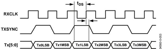
Figure 53. Tx[5:0] Port Full-Duplex Timing Diagram
