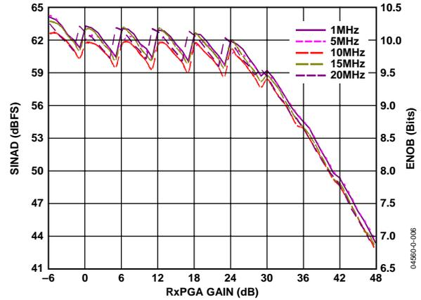
Figure 6. SINAD/ENOB vs. RxPGA Gain and Frequency
