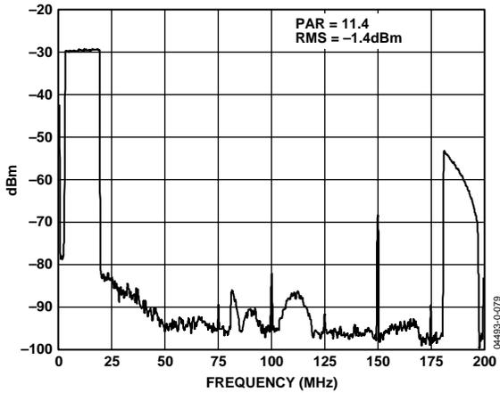
Figure 34. Wideband Spectral Plot of 88-Subcarrier OFDM Test Vector
