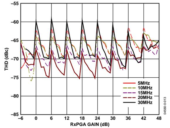
Figure 13. THD vs. RxPGA Gain and Frequency
