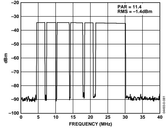
Figure 36. Spectral Plot of 111-Carrier OFDM Test Vector
