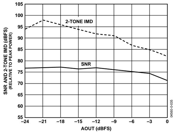
Figure 35. SNR and SFDR vs.  $P_{OUT}$
