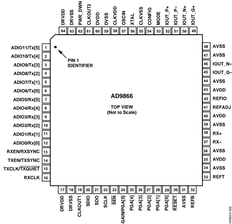
Figure 2. Pin Configuration
