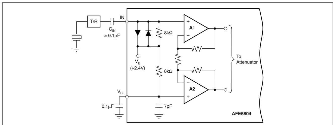
**Figure 99. LNA Channel (Simplified Schematic)**
