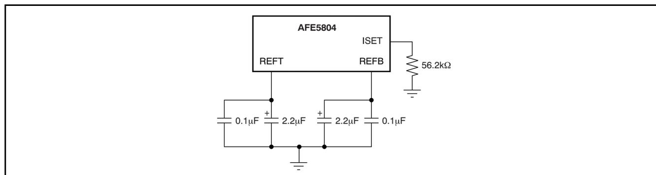
Figure 107. Suggested Decoupling on the Reference Pins
