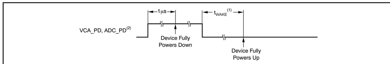
Power-up time shown is based on  $1\mu\text{F}$  bypass capacitors on the reference pins.  $t_{\text{WAKE}}$  is the time it takes for the device to wake up completely from power-down mode. The AFE5804 has two power-down modes: complete power-down mode and partial power-down mode.
