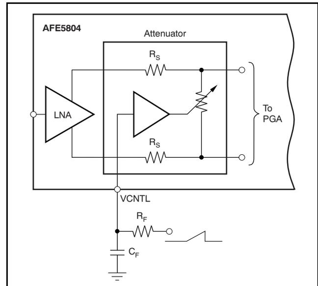
**Figure 101. External Filtering of the  $V_{CNTL}$  Input**
