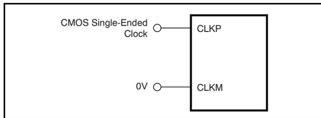
**Figure 103. Single-Ended Clock Driving Circuit (DIFF\_CLK = 0)**
