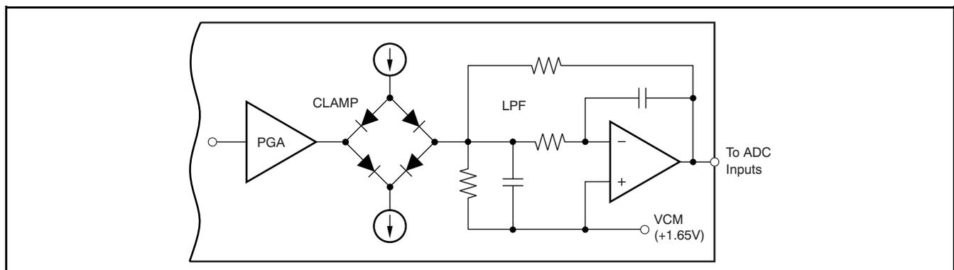
**Figure 98. Clamping Stage and Low-Pass Filter (Simplified Schematic)**
