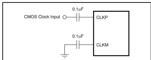
**Figure 106. Single-Ended Clock Driving Circuit When DIFF\_CLK = 1**
