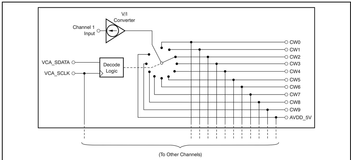
**Figure 91. Basic CW Cross-Point Switch Matrix Configuration**
