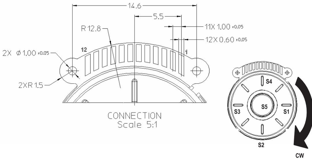
Figure 4. Electrical Connections
