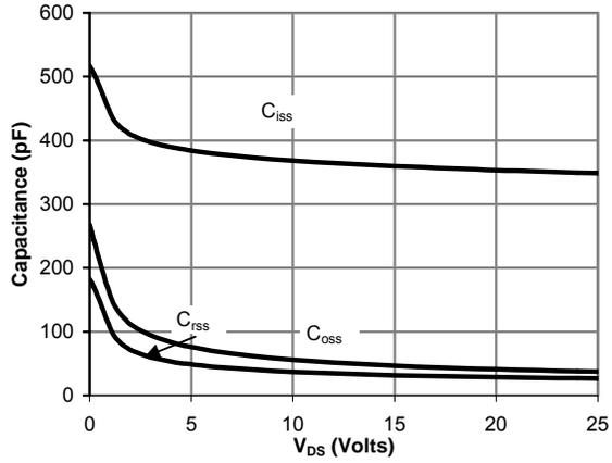
Figure 8: Capacitance Characteristics
