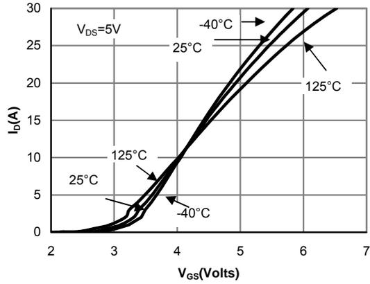
Figure 2: Transfer Characteristics
