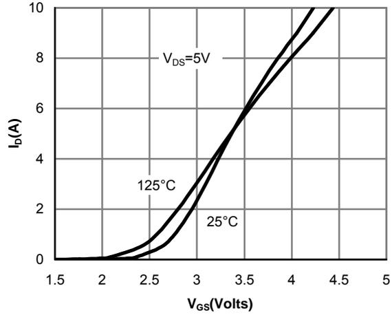
Figure 2: Transfer Characteristics
