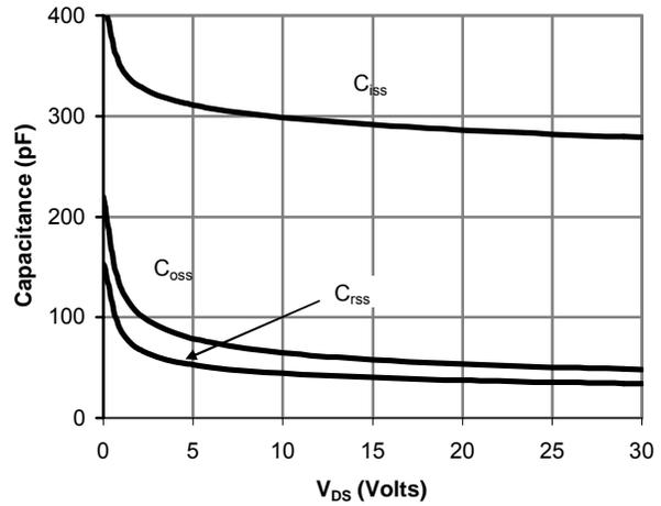
Figure 8: Capacitance Characteristics
