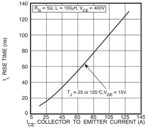
FIGURE 11, Current Rise Time vs Collector Current
