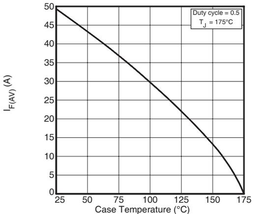
Figure 31. Maximum Average Forward Current vs. Case Temperature
