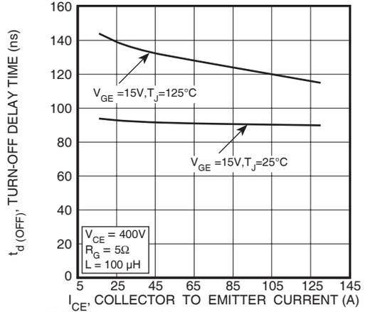
FIGURE 10, Turn-Off Delay Time vs Collector Current
