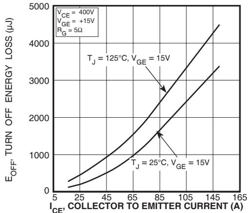
FIGURE 14, Turn Off Energy Loss vs Collector Current
