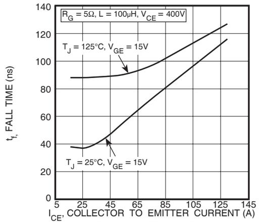
FIGURE 12, Current Fall Time vs Collector Current
