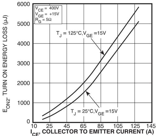
FIGURE 13, Turn-On Energy Loss vs Collector Current
