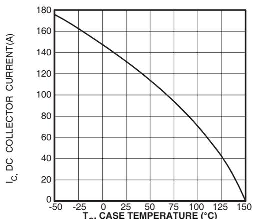
**FIGURE 8, DC Collector Current vs Case Temperature**
