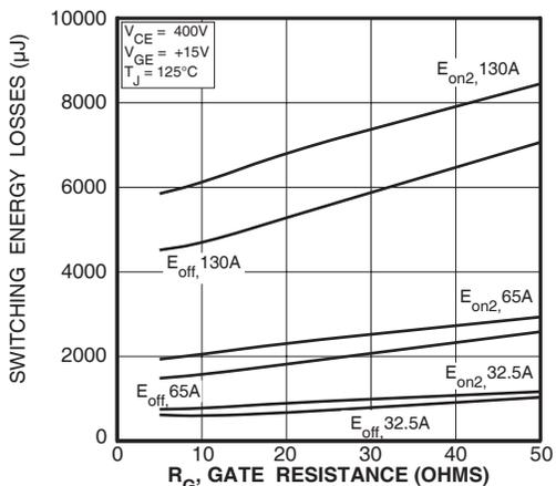
FIGURE 15, Switching Energy Losses vs. Gate Resistance
