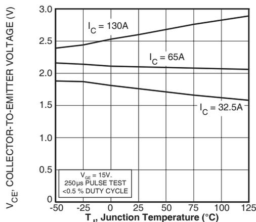
**FIGURE 6, On State Voltage vs Junction Temperature**
