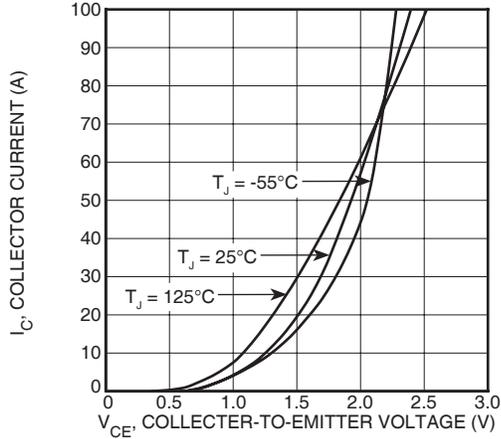
**FIGURE 1, Output Characteristics ( $T_J = 25^\circ\text{C}$ )**
