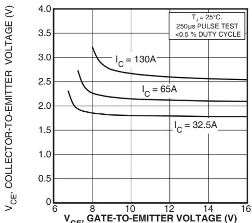
**FIGURE 5, On State Voltage vs Gate-to-Emitter Voltage**
