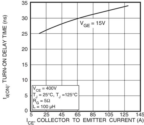
FIGURE 9, Turn-On Delay Time vs Collector Current
