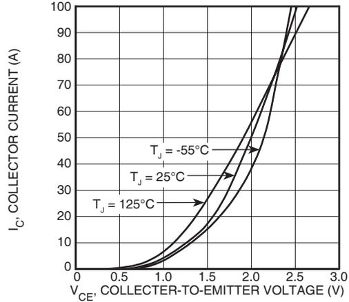
**FIGURE 2, Output Characteristics ( $T_J = 125^\circ\text{C}$ )**
