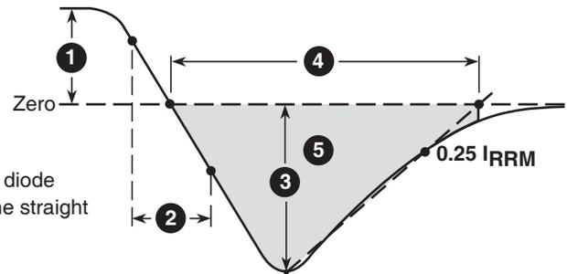
Figure 34, Diode Reverse Recovery Waveform and Definitions
