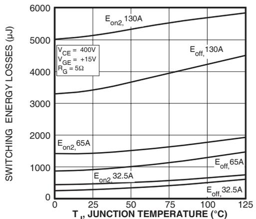
FIGURE 16, Switching Energy Losses vs Junction Temperature
