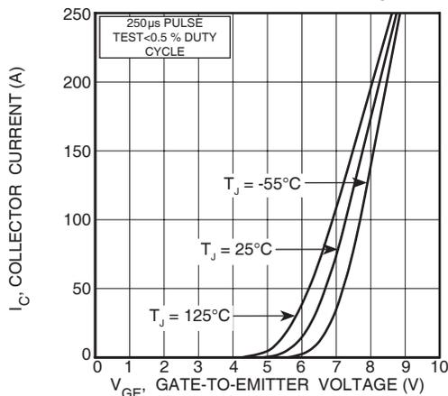
**FIGURE 3, Transfer Characteristics**
