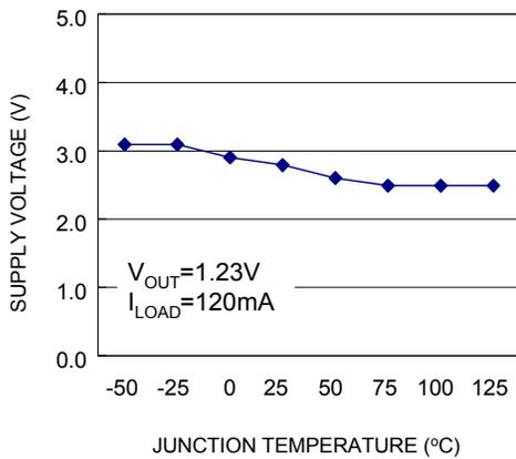
**ON/OFF Threshold Voltage**
