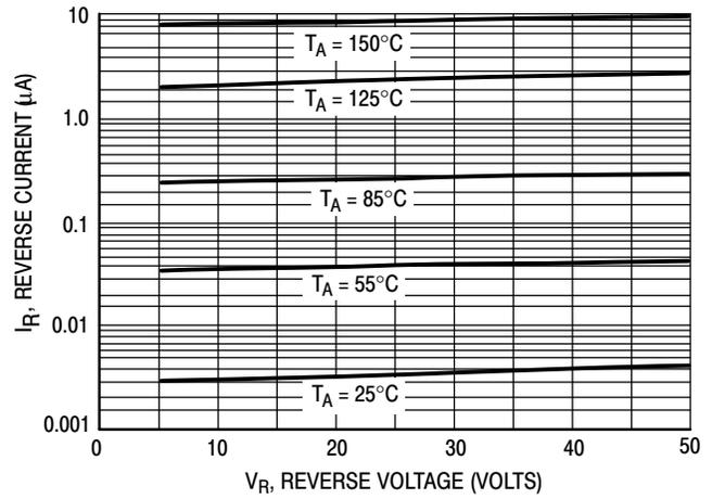
Figure 3. Leakage Current
