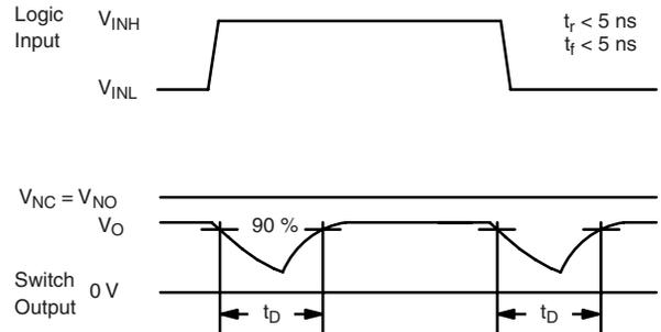
Figure 2. Break-Before-Make Interval
