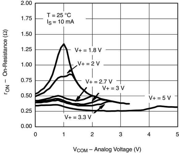
**r<sub>ON</sub> vs. V<sub>COM</sub> and Supply Voltage**
