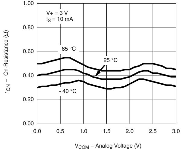
**r<sub>ON</sub> vs. Analog Voltage and Temperature**
