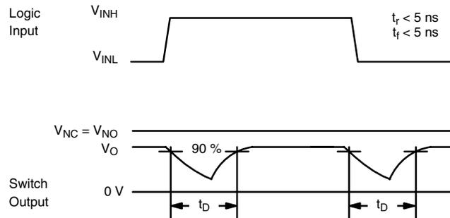
Figure 2. Break-Before-Make Interval
