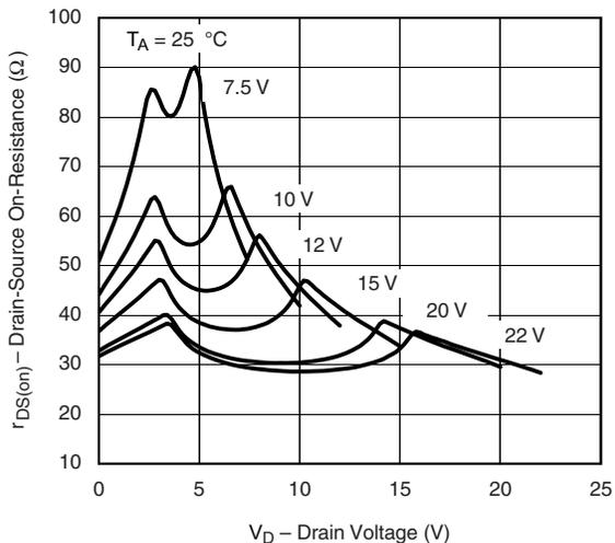
**r<sub>DS(on)</sub> vs. V<sub>D</sub> and Power Supply Voltage (V<sub>-</sub> = 0 V)**
