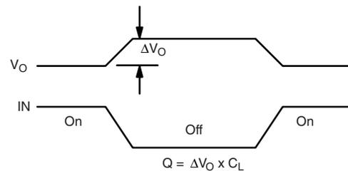
Figure 4. Charge Injection
