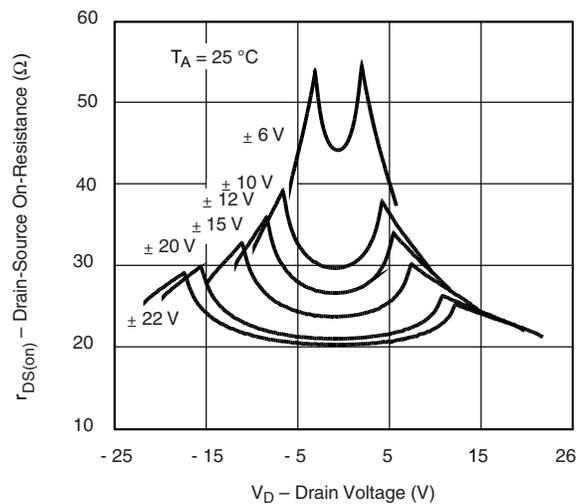
**r<sub>DS(on)</sub> vs. V<sub>D</sub> and Power Supply Voltage**
