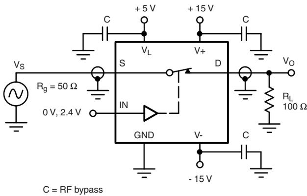
Figure 6. Insertion Loss
