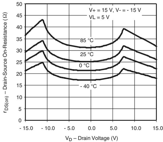
**r<sub>DS(on)</sub> vs. V<sub>D</sub> and Temperature**
