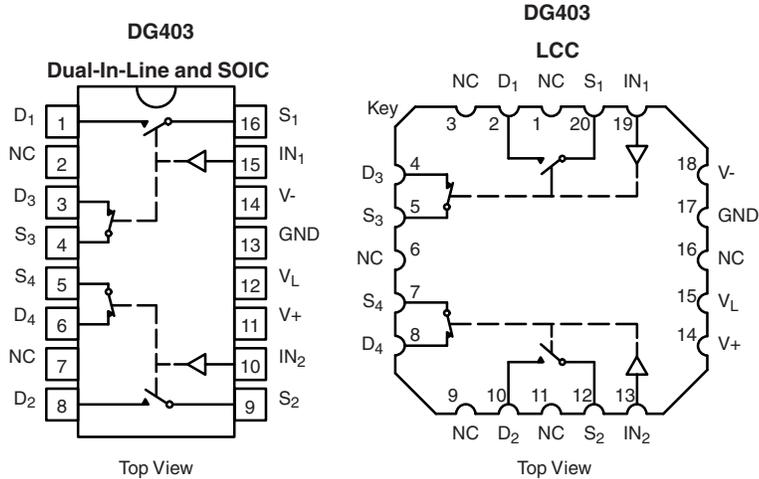
Two SPDT Switches per Package
