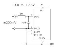
Measuring a single ended input voltage referenced to supply, i.e. the input voltage and the meter's power supply share the same 0V rail. Ensure solder link LREF is closed.
