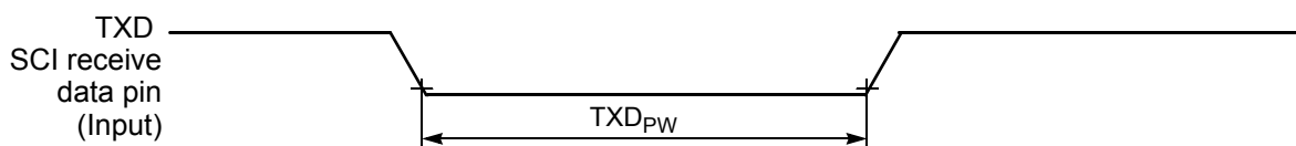
Figure 4-29 TXD Pulse Width
