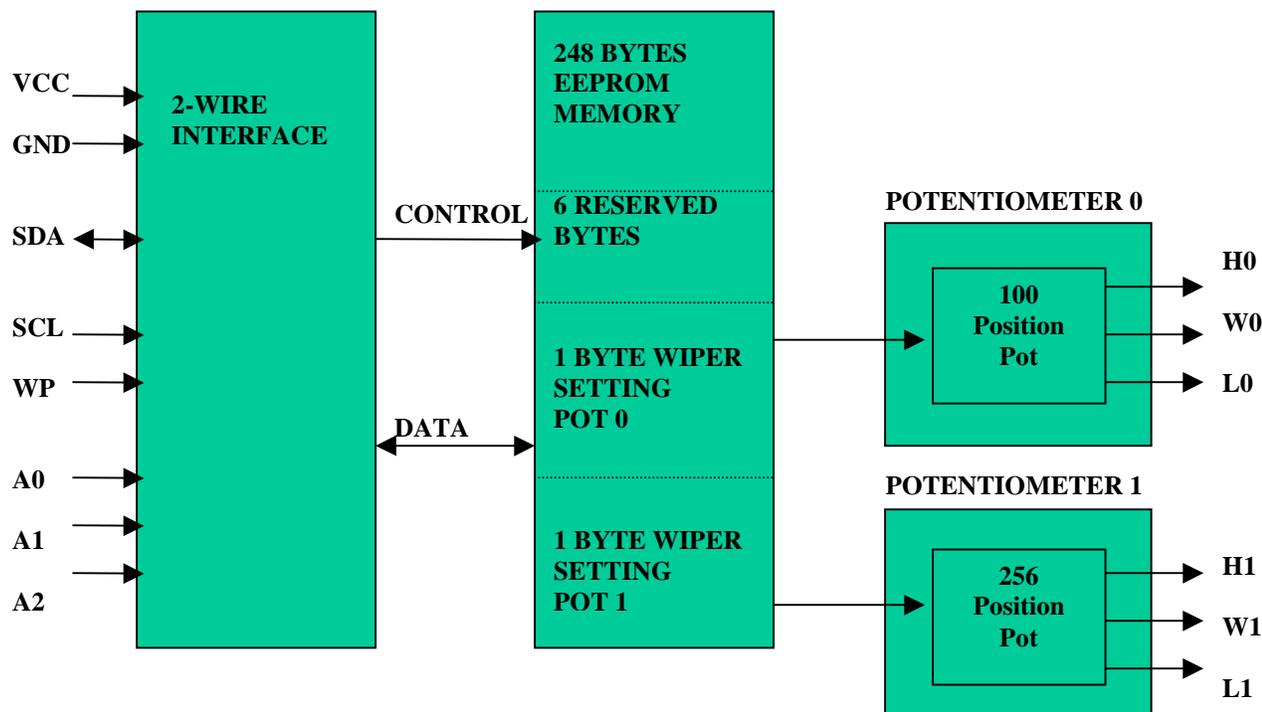
Up to eight DS1845s can be installed on a single 2-wire bus. Access to an individual device is achieved by using a device address that is determined by the logic levels of address pins  $A0$  through  $A2$ . Additionally, the DS1845 will operate from 3 volt or 5 volt supplies. Three package options are available: Flip Chip Package, 16-ball STPBGA and 14-pin TSSOP.
