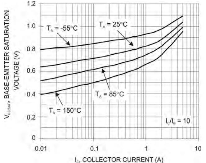
Fig. 6 Base-Emitter Saturation Voltage vs. Collector Current
