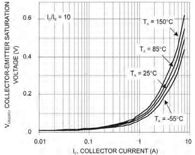
Fig. 4 Collector-Emitter Saturation Voltage vs. Collector Current
