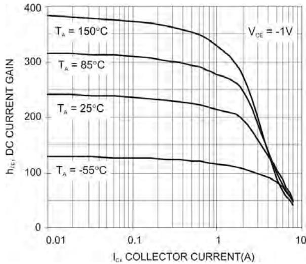
Fig. 3 Typical DC Current Gain vs. Collector Current
