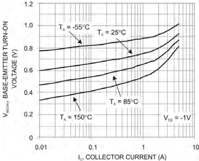
Fig. 5 Base-Emitter Turn-On Voltage vs. Collector Current
