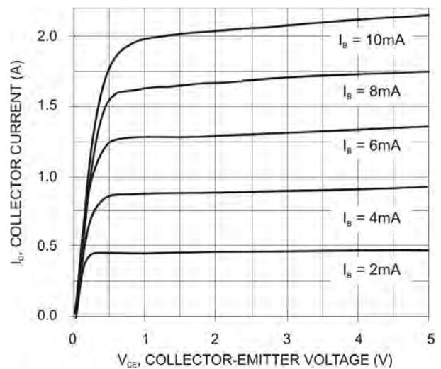
Fig. 2 Collector Current vs. Collector Emitter Voltage
