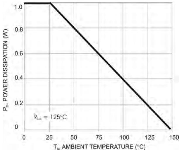
Fig. 1 Power Dissipation vs. Ambient Temperature (Note 3)
