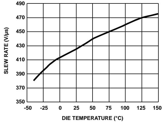
FIGURE 20. SLEW RATE vs TEMPERATURE
