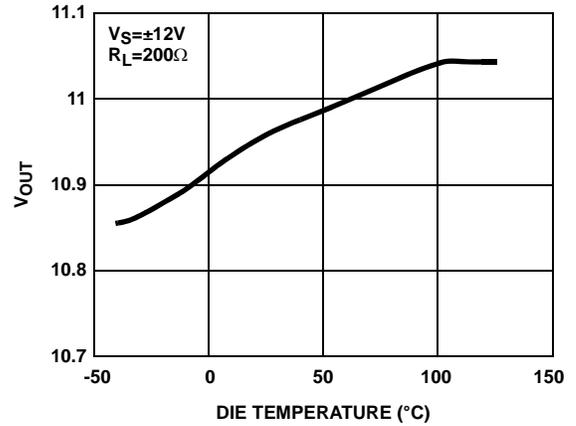
FIGURE 22. OUTPUT VOLTAGE vs TEMPERATURE
