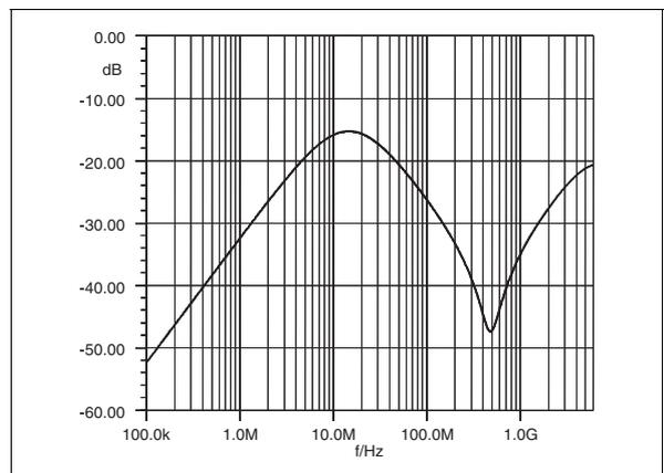
**Figure 5: ESD response to IEC61000-4-2 (+ 15kV air discharge) on one input V(in) and one output V(out)**
