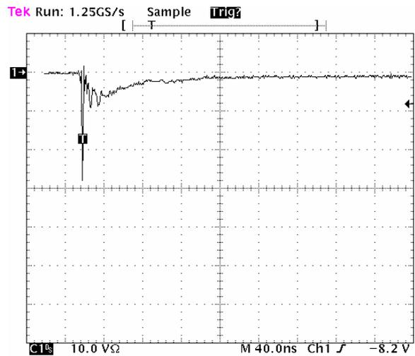
Figure 5. Negative 8 kV contact per IEC 6100-4-2 - ESD9X5.0ST5G
