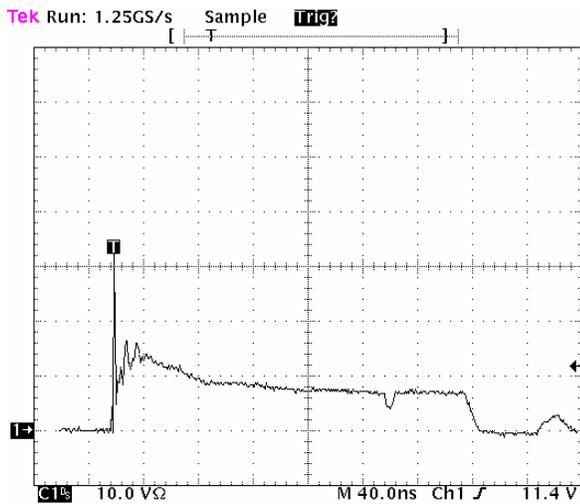
Figure 4. Positive 8 kV contact per IEC 6100-4-2 - ESD9X5.0ST5G
