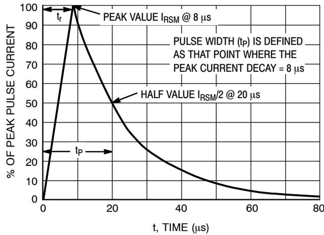
Figure 3. 8 X 20  $\mu$ s Pulse Waveform
