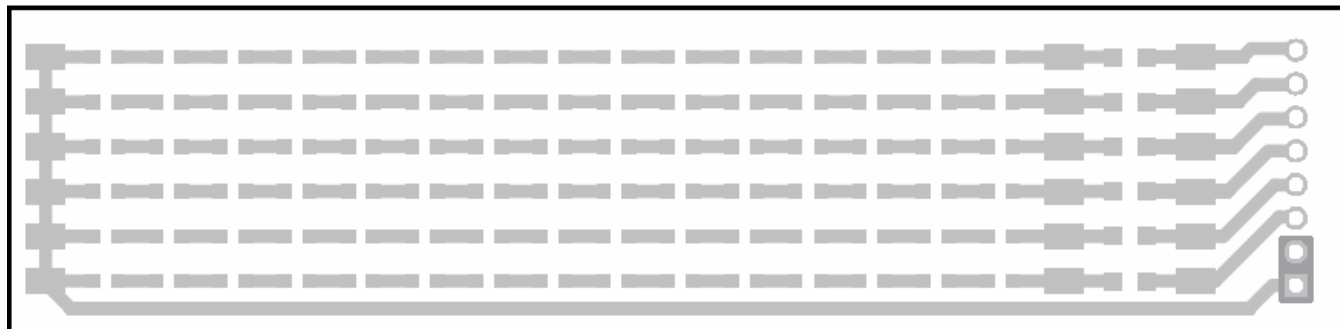
Figure 2—LED Board Top Layer
