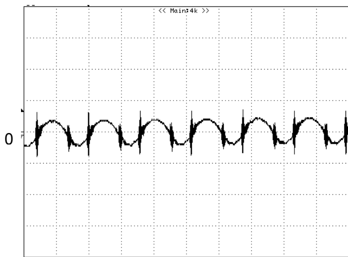
Figure 12: Input reflected ripple current, i_s , through a 12\mu\text{H} source inductor at nominal input voltage and rated load current (20 mA/div, 2 μs/div)
