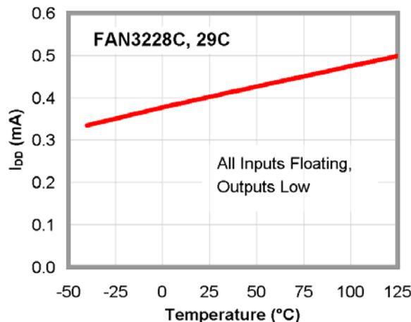
Figure 20.  $I_{DD}$  (Static) vs. Temperature<sup>(12)</sup>
