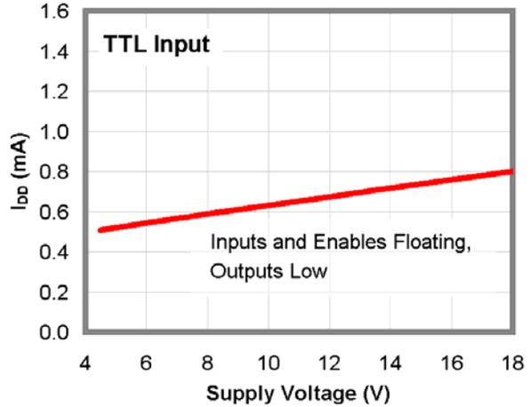
Figure 12.  $I_{DD}$  (Static) vs. Supply Voltage<sup>(12)</sup>
