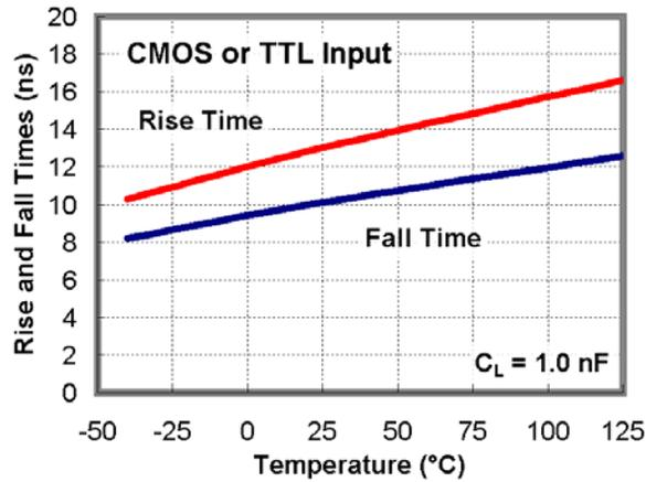
Figure 38. Rise and Fall Times vs. Temperature
