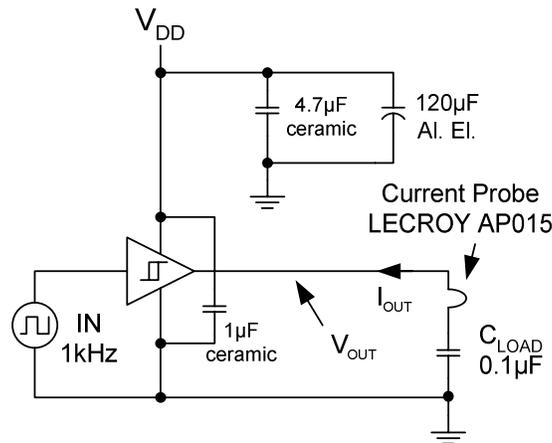
Figure 45. Quasi-Static  $I_{OUT}$  /  $V_{OUT}$  Test Circuit
