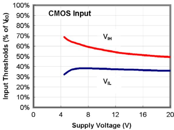
Figure 23. Input Threshold % vs. Supply Voltage
