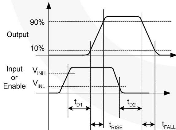
**Figure 9. Non-inverting**
