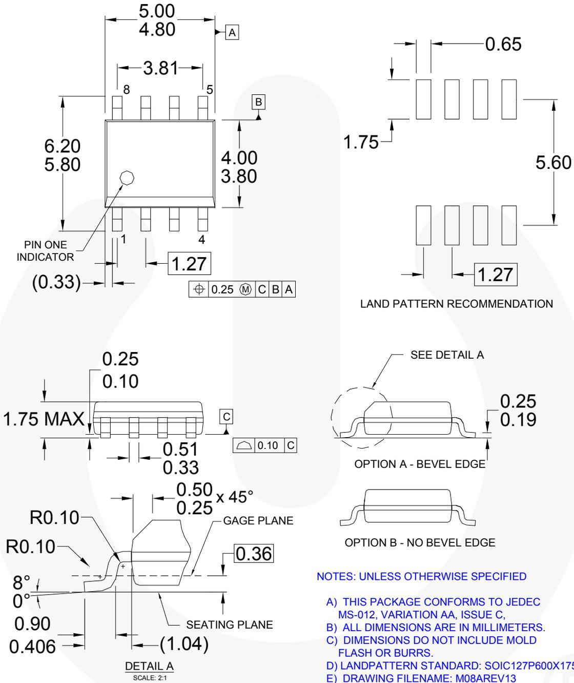
Figure 57. 8-Lead SOIC
