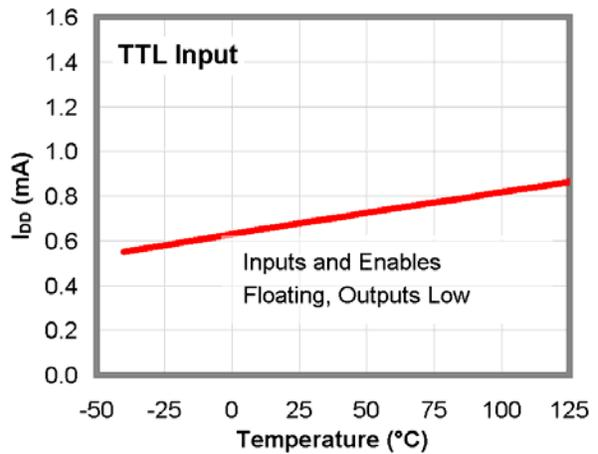
Figure 19.  $I_{DD}$  (Static) vs. Temperature<sup>(12)</sup>
