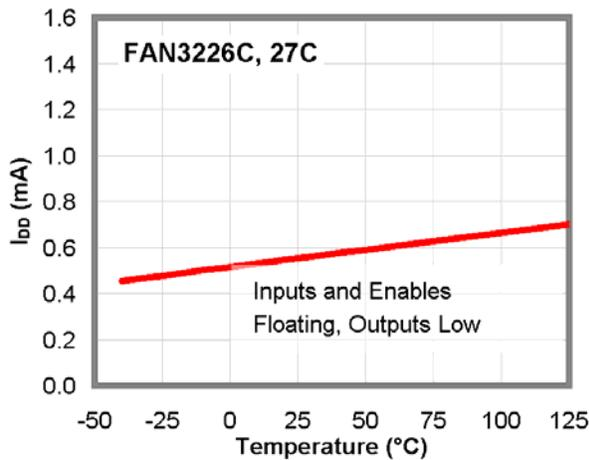
Figure 18.  $I_{DD}$  (Static) vs. Temperature<sup>(12)</sup>
