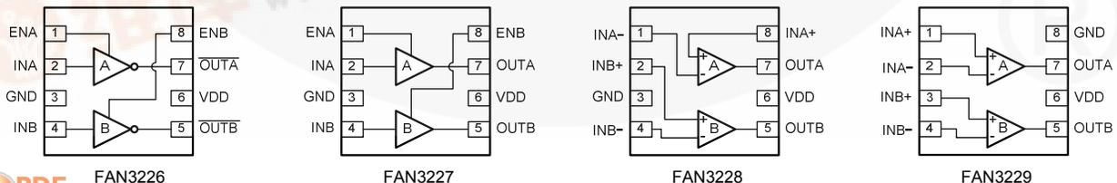
Figure 1. Pin Configurations
