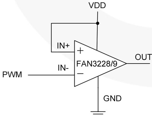
**Figure 50. Dual-Input Driver Enabled, Inverting Configuration**
