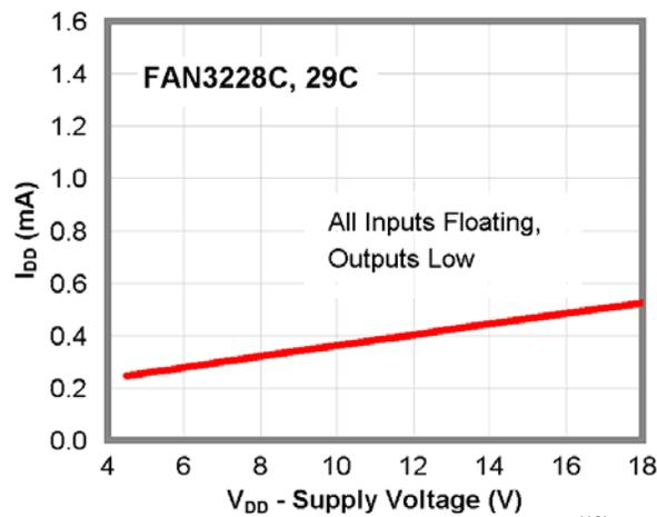
Figure 13.  $I_{DD}$  (Static) vs. Supply Voltage<sup>(12)</sup>
