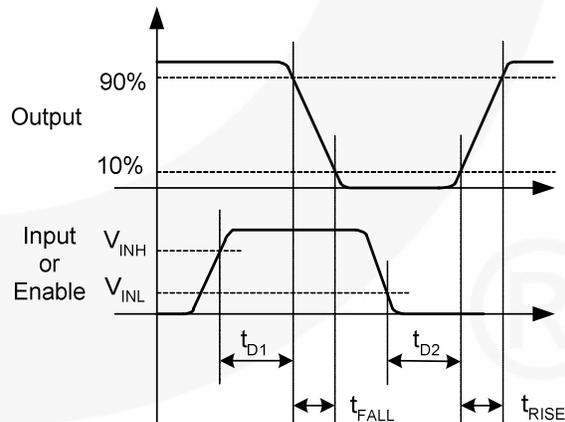
**Figure 10. Inverting**
