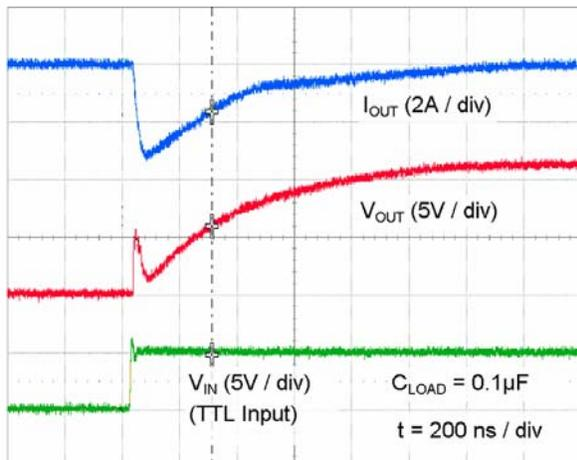
Figure 41. Quasi-Static Source Current with  $V_{DD}=12V$
