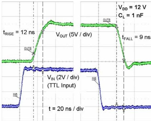
Figure 39. Rise/Fall Waveforms with 1nF Load
