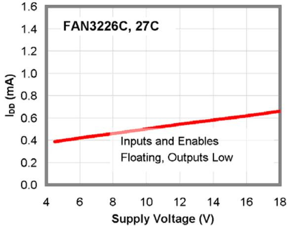
Figure 11.  $I_{DD}$  (Static) vs. Supply Voltage<sup>(12)</sup>
