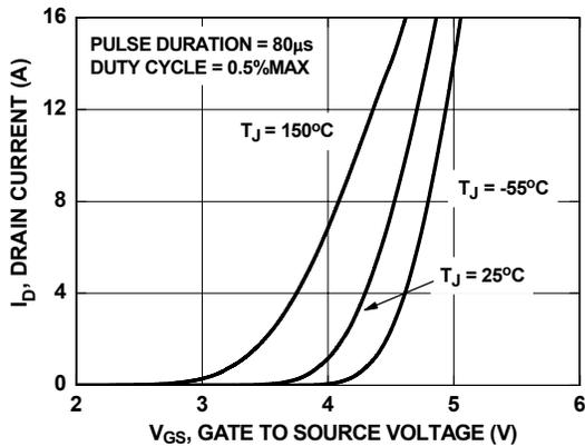
Figure 5. Transfer Characteristics
