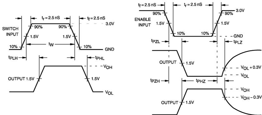
FIGURE 2. AC Waveforms
