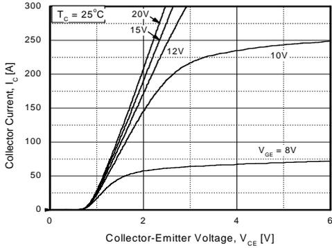
Figure 6. Typical Output Characteristics
