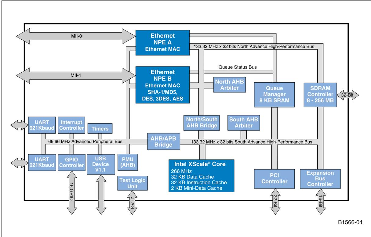
Figure 4. Intel® IXP421 Network Processor Block Diagram
