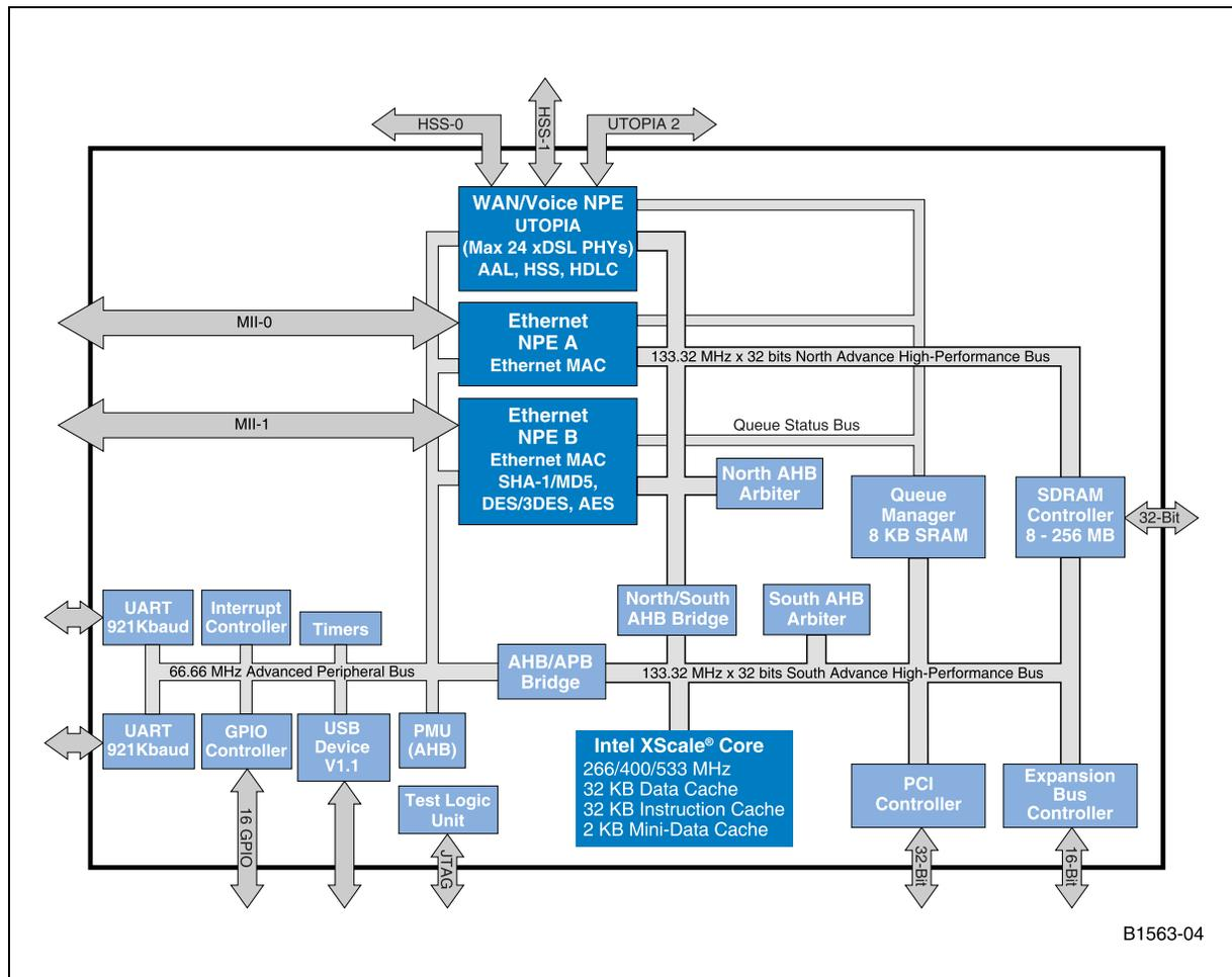
Figure 2. Intel® IXP423 Network Processor Block Diagram
