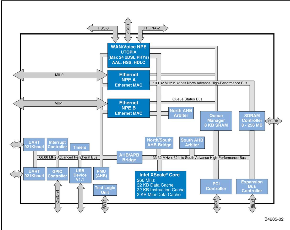
Figure 3. Intel® IXP422 Network Processor Block Diagram
