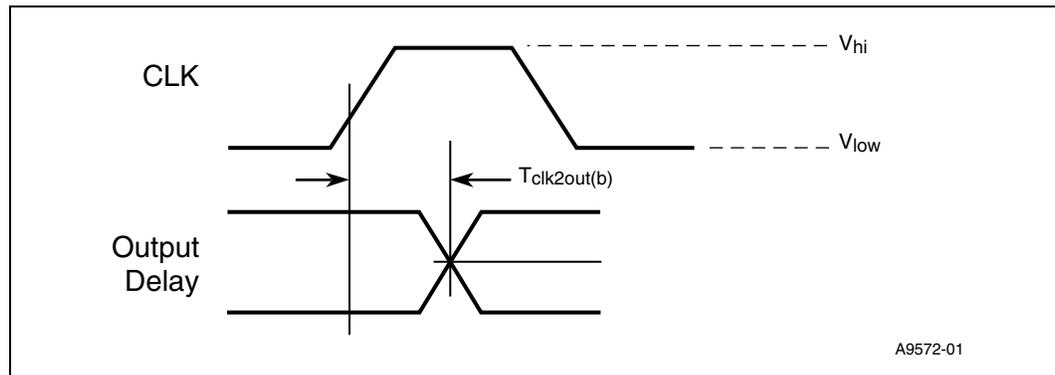
**Note:**  $V_{HI} = 0.6 V_{CC}$  and  $V_{LOW} = 0.2 V_{CC}$
