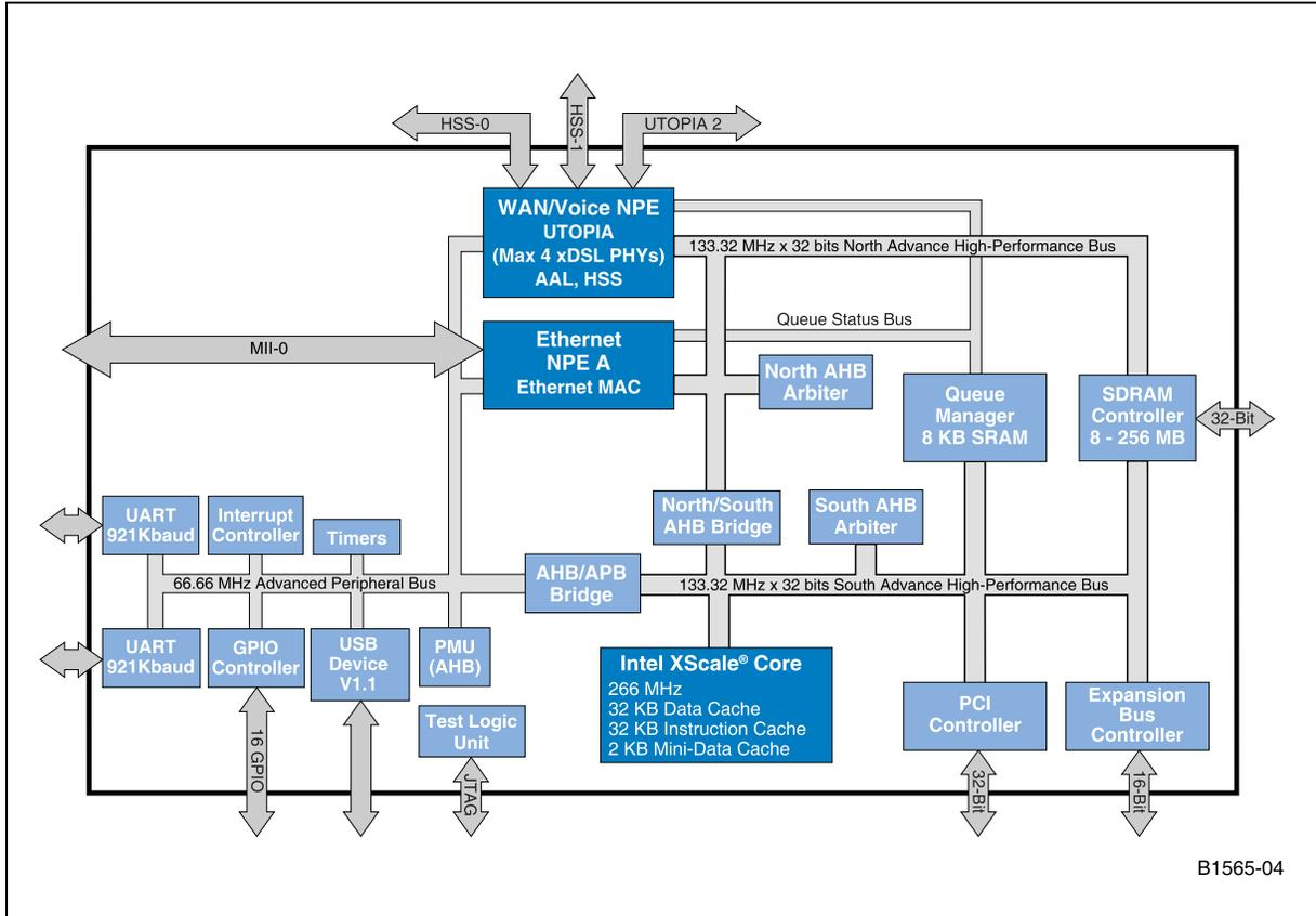
Figure 5. Intel® IXP420 Network Processor Block Diagram
