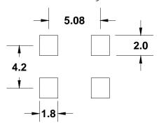
Note: XPRESSO HCMOS XOs are designed to fit or industry standard, 4 pad, layouts.
