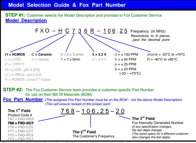
This example, FXO-HC736R-106.25 = HCMOS Output, Ceramic 7 x 5mm Package, 3.3V, ±25 PPM Stability, -40 to +85°C Temperature Range, at 106.25 MHz
