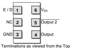
NOTE: XPRESSO LVPECL XOs are designed to fit on Industry Standard, 6 pad layouts
