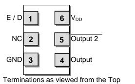
NOTE: XPRESSO LVPECL XOs are designed to fit on Industry Standard, 6 pad layouts
