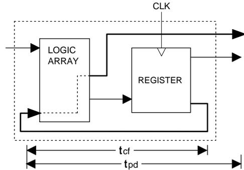
**f<sub>max</sub> with Internal Feedback 1/(t<sub>su</sub>+t<sub>cf</sub>)**
