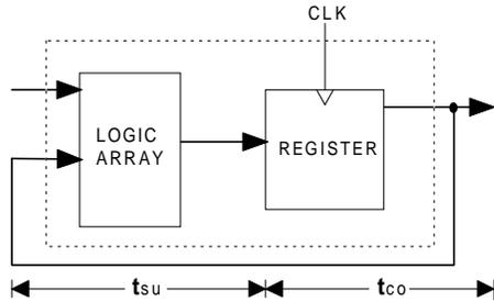
**f<sub>max</sub> with External Feedback 1/(t<sub>su</sub>+t<sub>co</sub>)**
