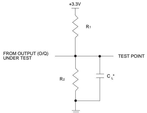
\*C<sub>L</sub> INCLUDES TEST FIXTURE AND PROBE CAPACITANCE
