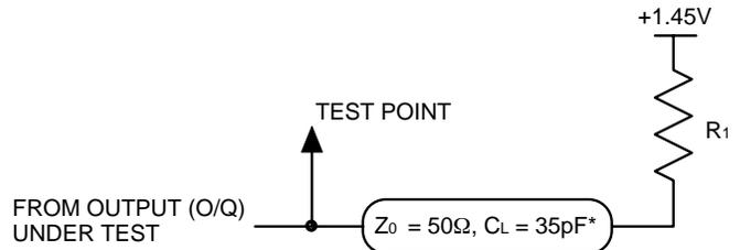
\*C<sub>L</sub> INCLUDES TEST FIXTURE AND PROBE CAPACITANCE
