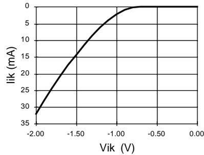
**GAL16LV8C: Typical AC and DC Characteristic Diagrams**
