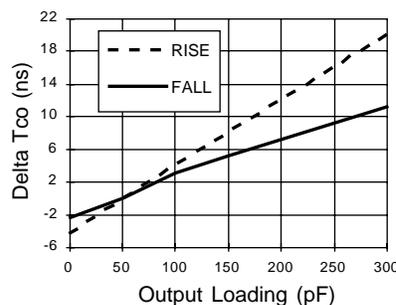
**GAL16LV8D: Typical AC and DC Characteristic Diagrams**
