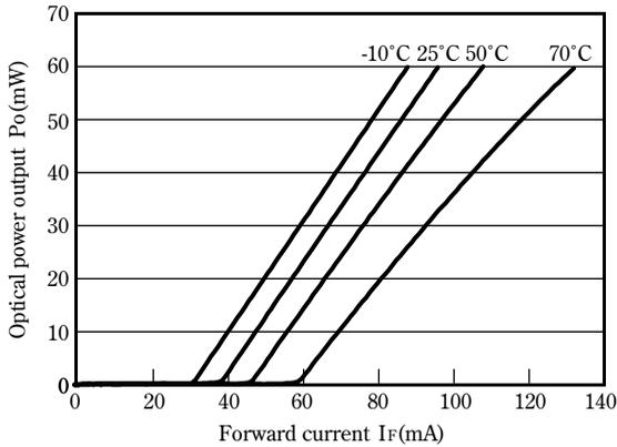
Optical power output - Forward current [Pulse]
