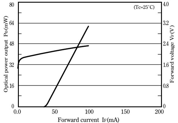
Forward voltage - Forward current [Pulse]
