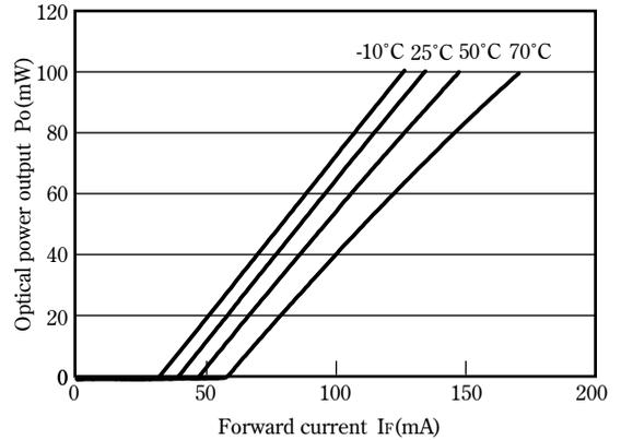
Case temperature dependence of threshold current [CW]
