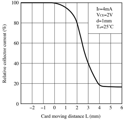
**Fig.14 Test Condition for Distance & Detecting Position Characteristics**
