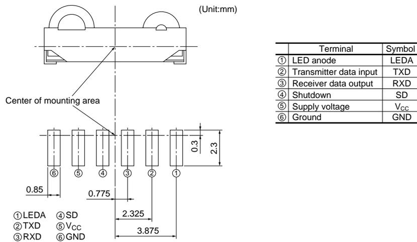
**Fig.10 Recommended Size of Solder Creamed Paste (Reference)**
