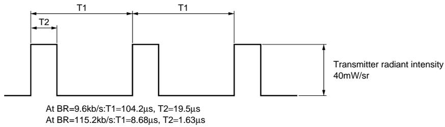
Fig.4 Output Waveform Specification (Receiver side)
