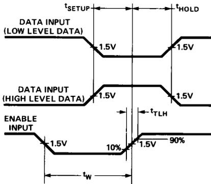
Figure 1. Timing Diagram.
