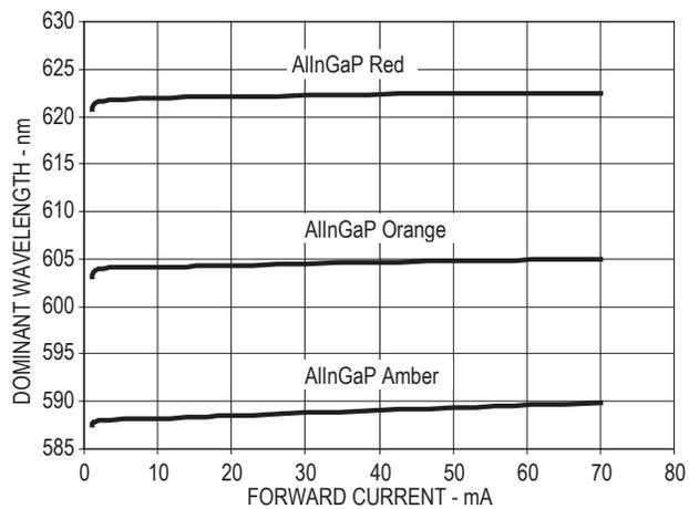
**Figure 7. Dominant Wavelength Vs. Forward Current.**
