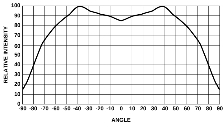
Figure 5d. Relative intensity vs. angle for HSMx-C120.
