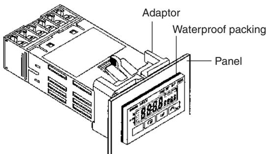
The H8GN's panel surface is water-resistive (conforming to NEMA 4X (indoors) and IP66). In order to prevent the internal circuit from water penetration through the space between the Counter and operating panel, attach a rubber packing (provided with the H8GN) between the Counter and operating panel and secure the rubber packing with the Y92F-34 Flush-mounting Adaptor.
