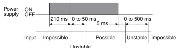
Turn the power ON and OFF using a relay with a rated capacity of 15 A minimum to prevent contact deterioration due to inrush current caused by turning the power ON and OFF.
