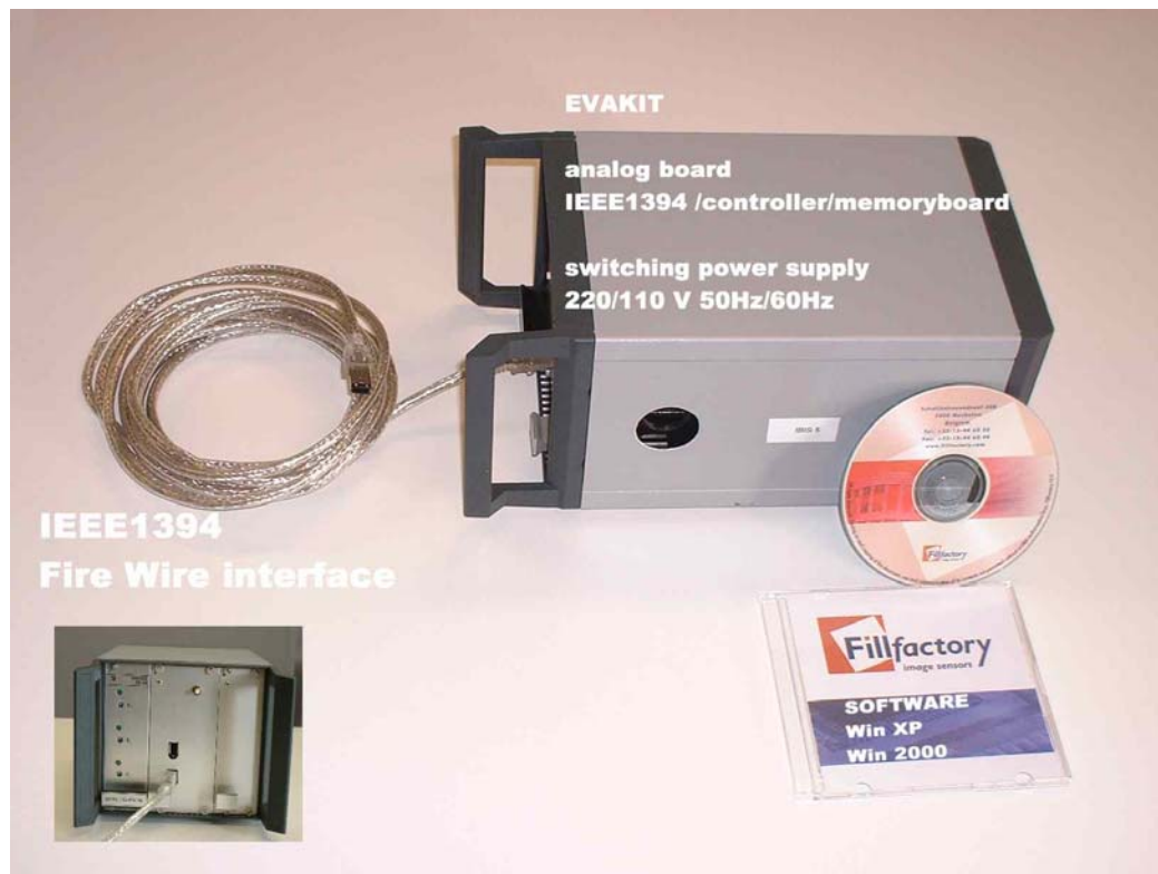
Figure 36: Content of the IBIS4 evaluation kit
