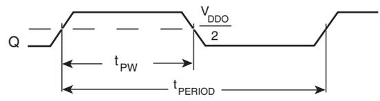
$$odc = \frac{t_{PW}}{t_{PERIOD}} \times 100\%$$
