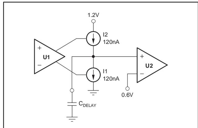
**Figure 6. Simplified Model of the Comparator 2 Delay Circuit**
