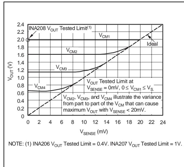
**Figure 4. Example for Low  $V_{SENSE}$  Case 2 (INA208, Gain = 100)**
