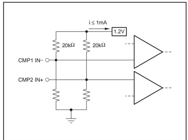
Figure 9. Limit Current Into Reference  $\leq 1mA$
