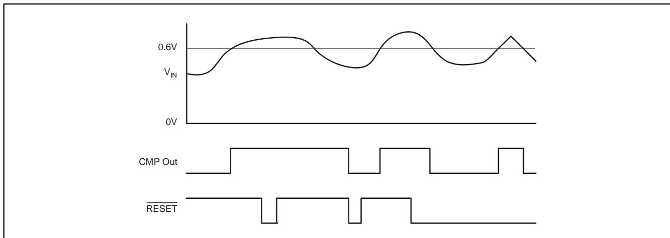
**Figure 7. Comparator 1 Latching Capability**
