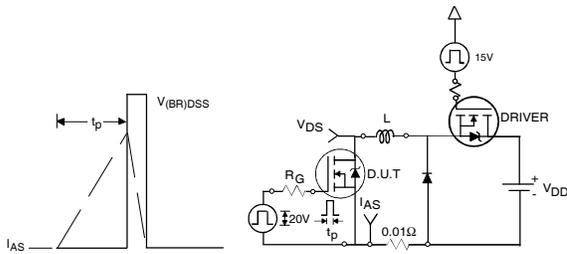
**Fig 15a&b.** Unclamped Inductive Test circuit and Waveforms
