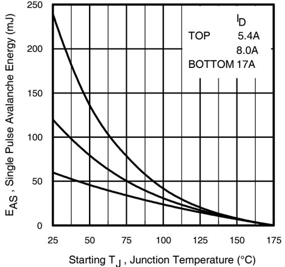
**Fig 16.** Maximum Avalanche Energy vs. Drain Current
