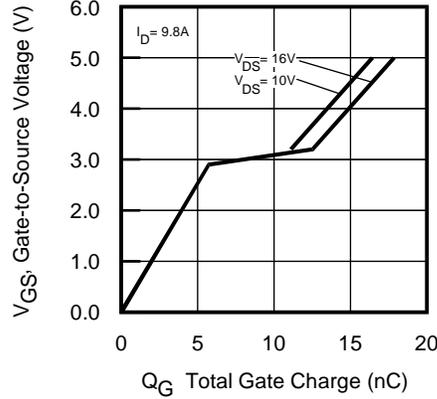
**Fig. 10.** Gate-to-Source Voltage vs Typical Gate Charge
