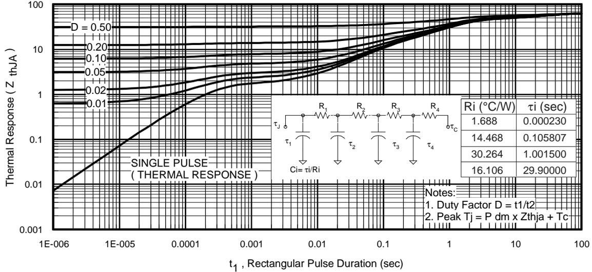
Fig 25. Maximum Effective Transient Thermal Impedance, Junction-to-Ambient
