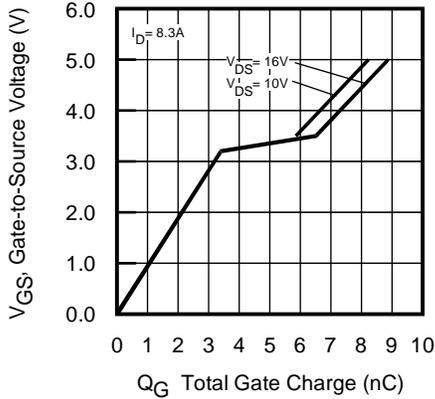
**Fig. 9.** Gate-to-Source Voltage vs Typical Gate Charge
