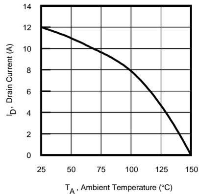
**Fig 20. Maximum Drain Current vs. Ambient Temperature**
