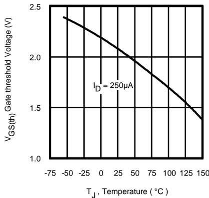
**Fig 21. Threshold Voltage vs. Temperature**
