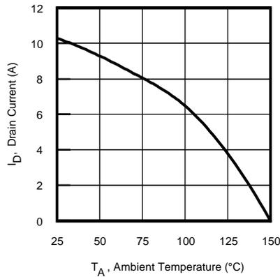
**Fig 19. Maximum Drain Current vs. Ambient Temperature**
