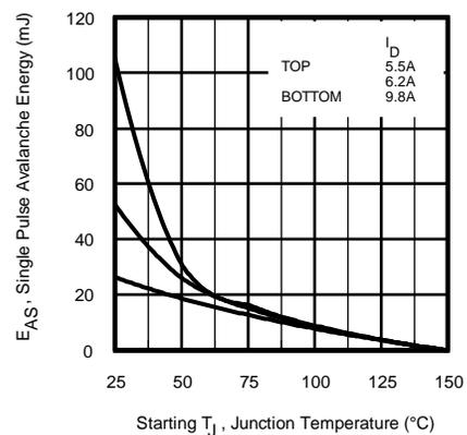
**Fig 24. Maximum Avalanche Energy vs. Drain Current**
