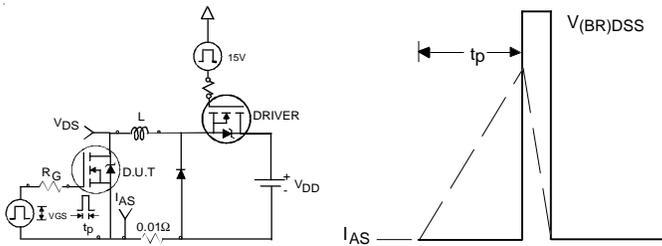
Fig 26. Unclamped Inductive Test Circuit and Waveform
