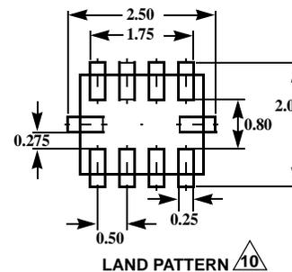
Thin Dual Flat No-Lead Plastic Package (TDFN)
