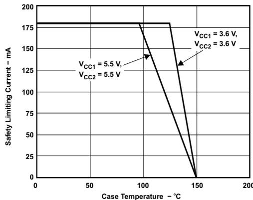
Figure 7.  $\theta_{JC}$  THERMAL DERATING CURVE per IEC 60747-5-2
