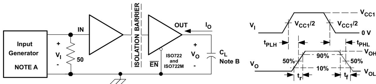
Figure 1. Switching Characteristic Test Circuit and Voltage Waveforms
