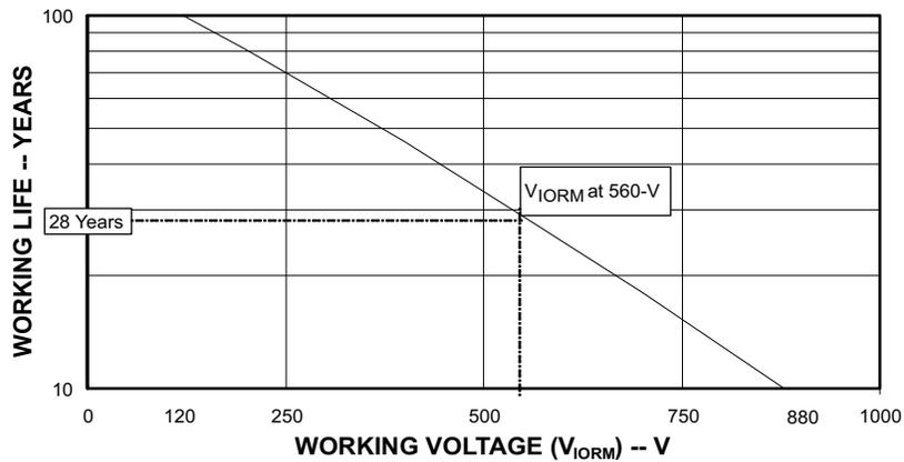
Figure 10. Time Dependant Dielectric Breakdown Testing Results
