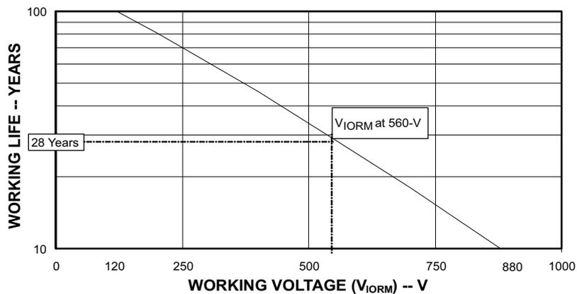
Figure 14. Time Dependant Dielectric Breakdown Testing Results
