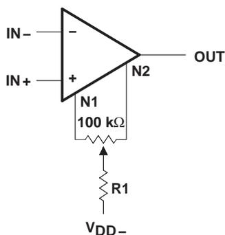
NOTE A:  $R_1 = 5.6\text{ k}\Omega$  for offset voltage adjustment of  $\pm 10\text{ mV}$ .
