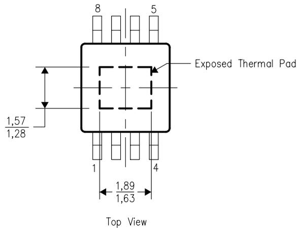
NOTE: All linear dimensions are in millimeters
