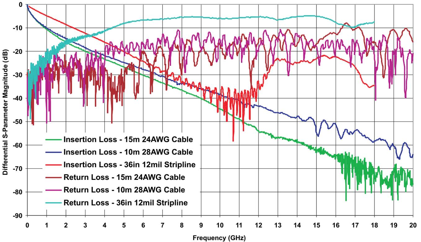
**Figure 6. Typical Differential S-Parameter Characteristics of Interconnect Lines**
