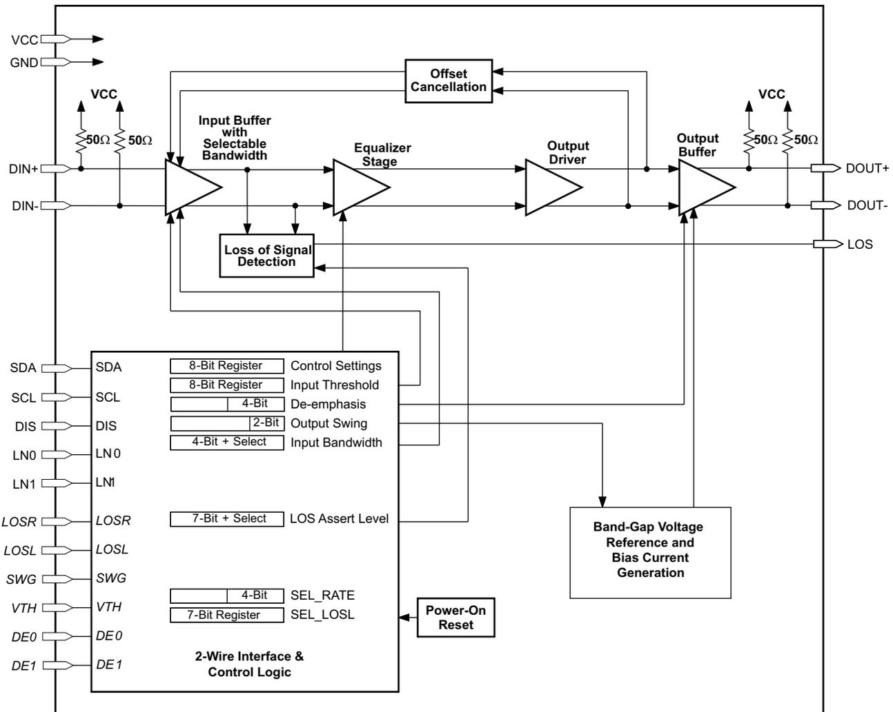
Figure 1. Simplified Block Diagram of the TLK1101E
