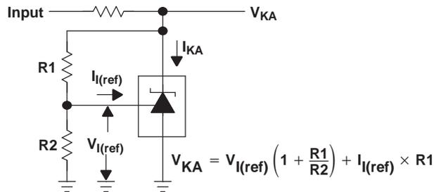
Figure 2. Test Circuit for  $V_{(KA)} > V_{ref}$
