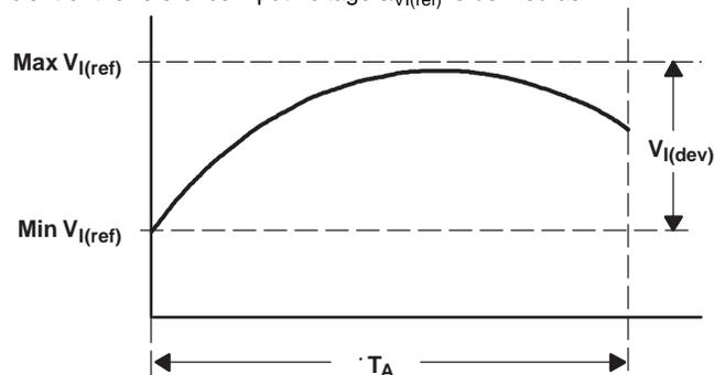
$\alpha_{V_{I(ref)}}$  is positive or negative, depending on whether minimum  $V_{I(ref)}$  or maximum  $V_{I(ref)}$ , respectively, occurs at the lower temperature.
