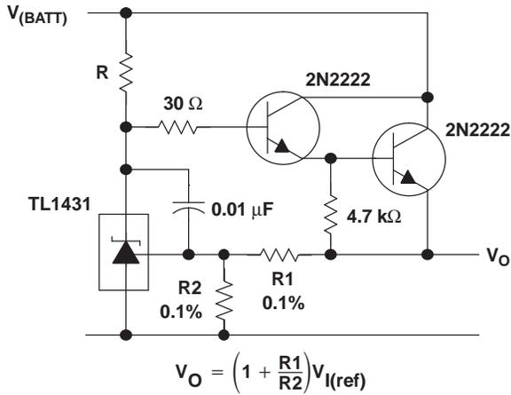
A. R should provide cathode current  $\geq 1$  mA to the TL1431 at minimum  $V_{(BATT)}$ .
