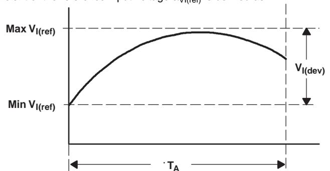
$\alpha_{V_{I(\text{ref})}}$  is positive or negative, depending on whether minimum  $V_{I(\text{ref})}$  or maximum  $V_{I(\text{ref})}$ , respectively, occurs at the lower temperature.
