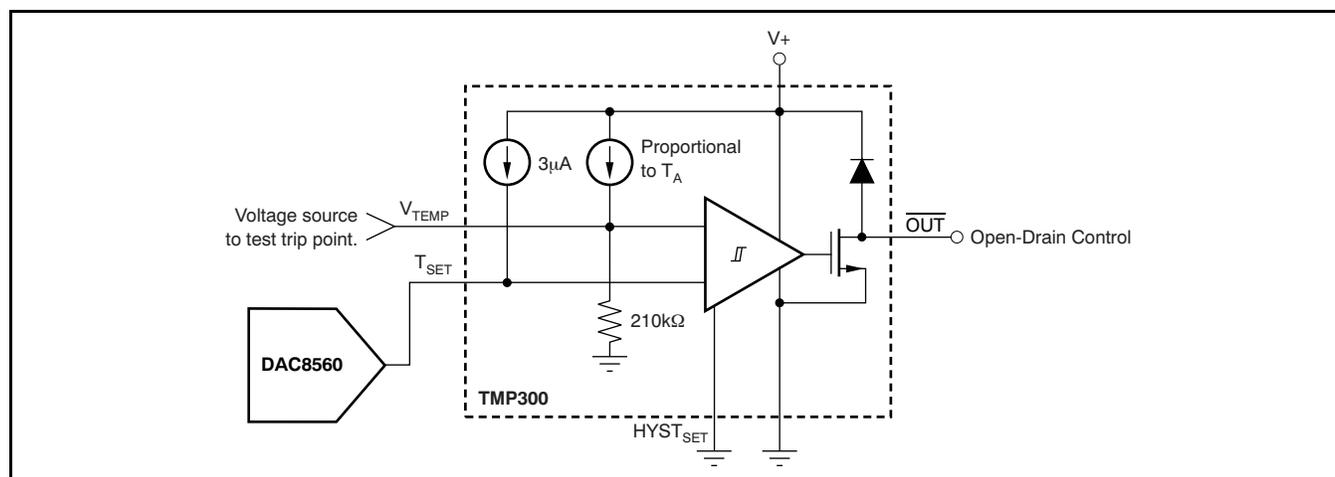
Figure 11. DAC Generates the Voltage-Driving  $T_{SET}$  Pin
