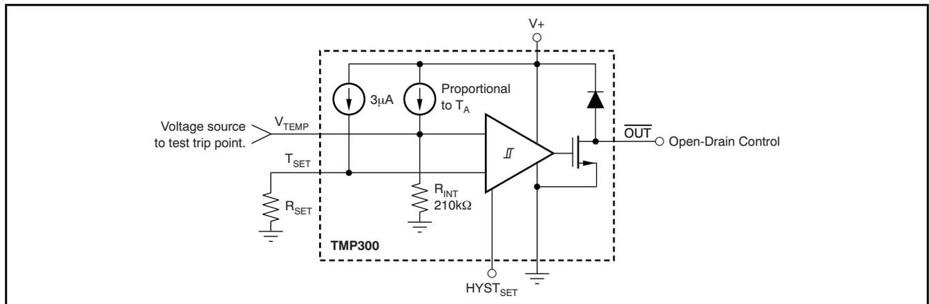
**Figure 8. Applying Voltage to Trip Digital Output**
