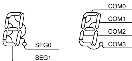
Figure 13-6 Example of COM, SEG Pin Connection (1/4 Duty)
